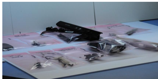
Figure 11. Subassemblies are bagged and tagged. The Kinect took a total of ten phases to dismantle.
